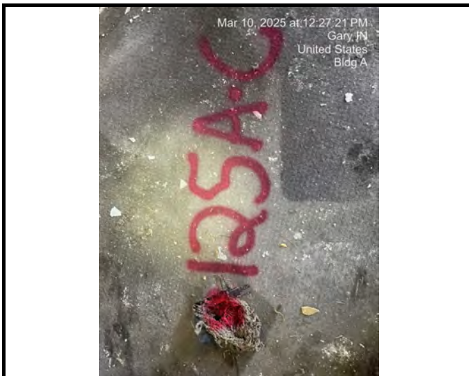
Sample # A-3-125 Flooring - Linoleum with Paper Backing-White
