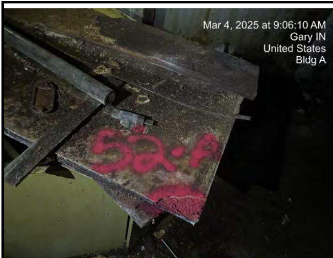
Sample # A-52-Bas Flooring - Linoleum with Paper Backing
