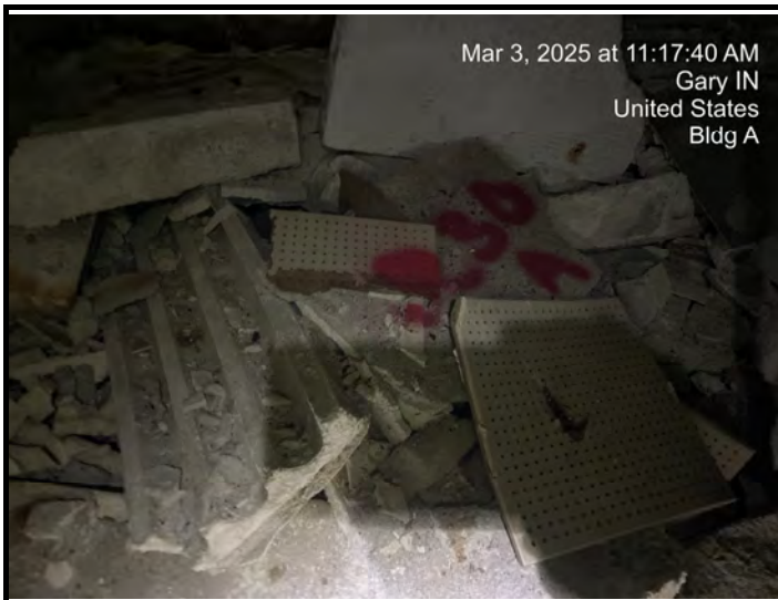
Sample # A-30-Bas Ceiling Tile - 1X1 w/Glue Pod, White with Dot pattern
