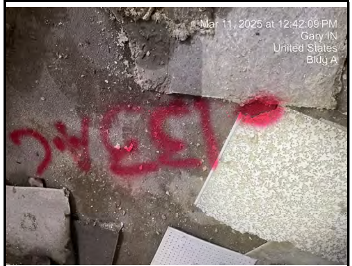
Sample # A-4-133 Ceiling Panel - 2X2, White with Gouges
