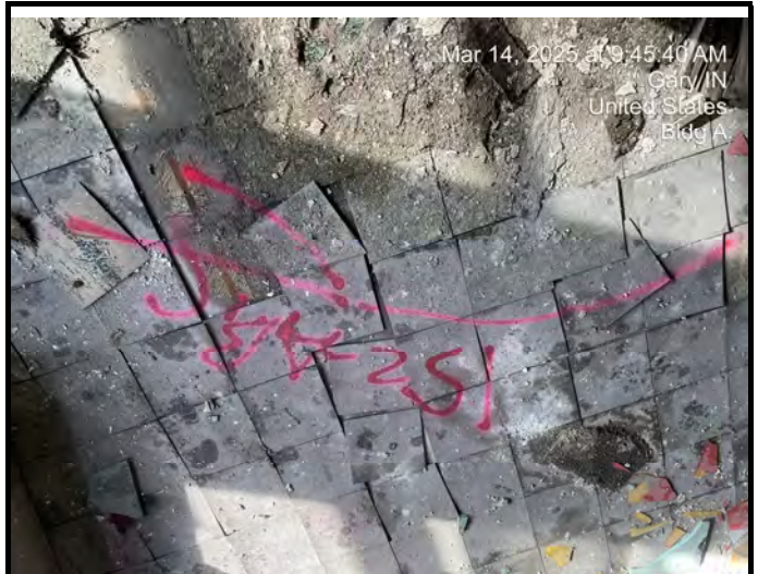
Sample # A-R-152 Flooring- Black with Green Dots - 12X12 Floor Tile with Glue
