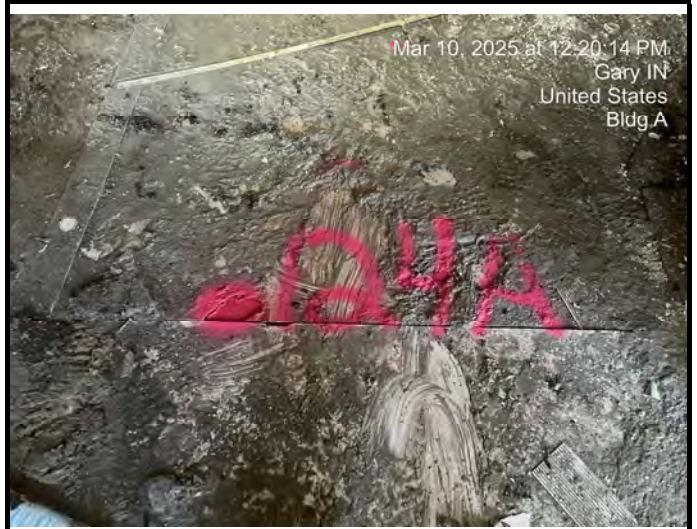
Sample # A-3-124 Flooring - Linoleum with Paper Backing-Beige with Red, White, Blue Speckles
